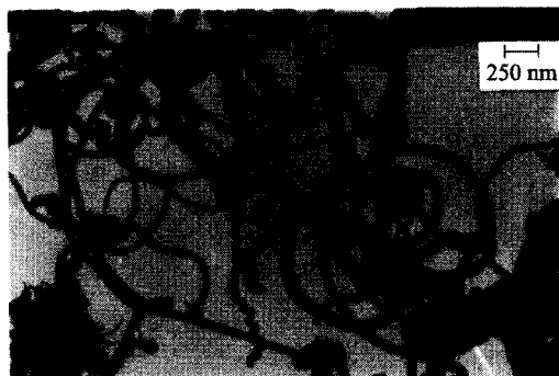
Fig. 6 TEM image of carbon filament grown over LaCoO 3 pre-reduced at 700°C.
